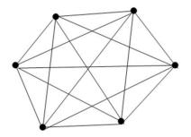
To connect 'N' Points the number of Links are required are :  $\frac{n(n-1)}{2}$
