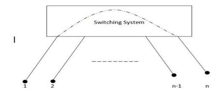
Telephone Exchange/Switching is a system which will provide a temporary connection between any two telephones when required therefore to connect 'n' telephones, it requires only 'n – links'
